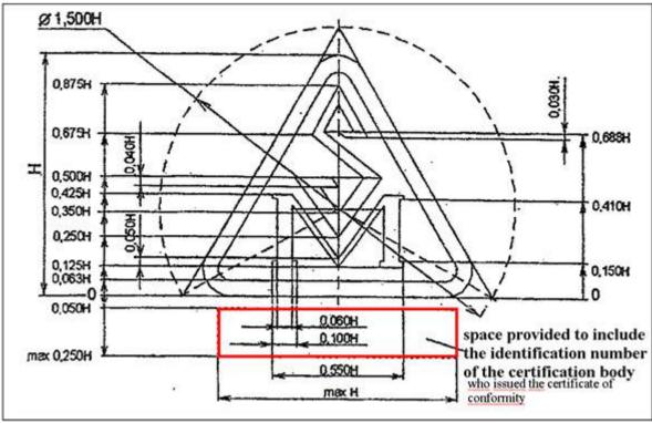
Figure 2. The dimensions of the national conformity label SM
